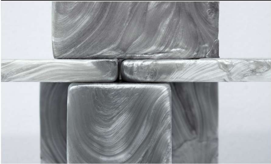
Plasticiet stretches recycled plastic like taffy for Mother of Pearl furniture
